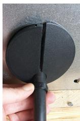
Fit the bushing over the cord and slide into place, flush with the new plug.
