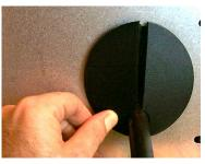
Fit the plug over the powercord and slide into place, ensuring the plug
